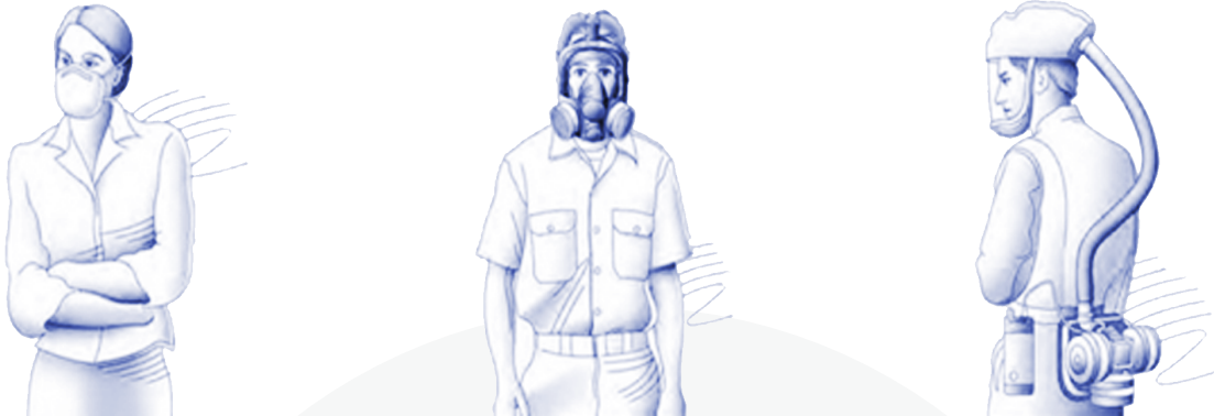
The workers shown above are wearing a NIOSH-approved N95 filtering facepiece respirator (left), a full facepiece elastomeric respirator (center), and a loose-fitting powered air-purifying respirator (PAPR) (right).
